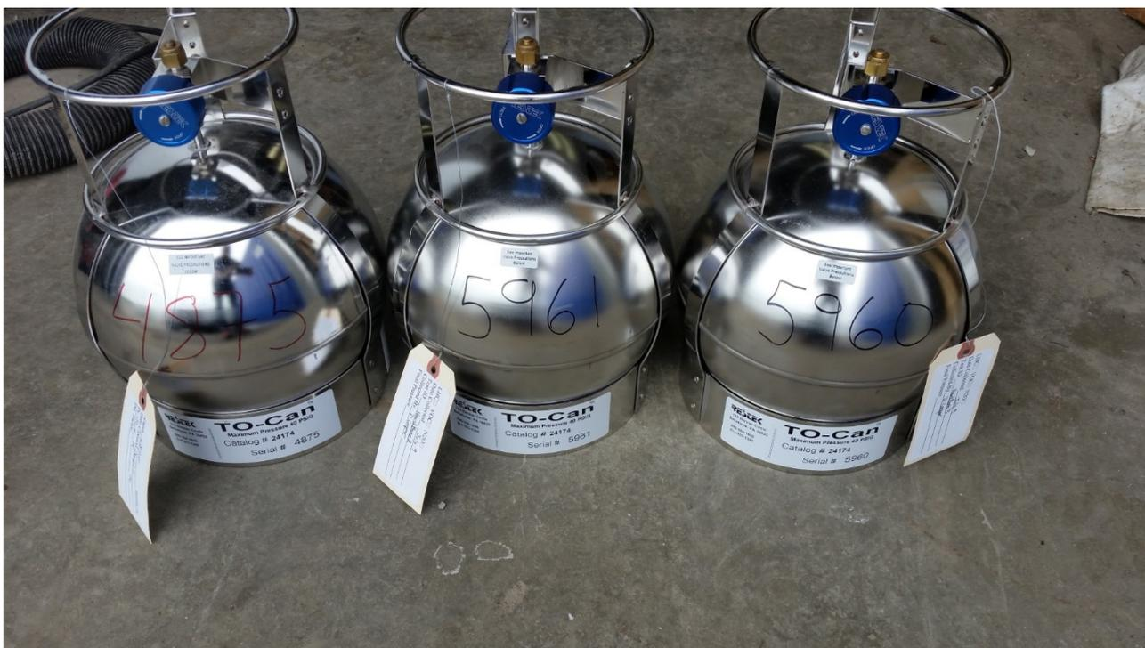
Figure 92: Sampling canisters
