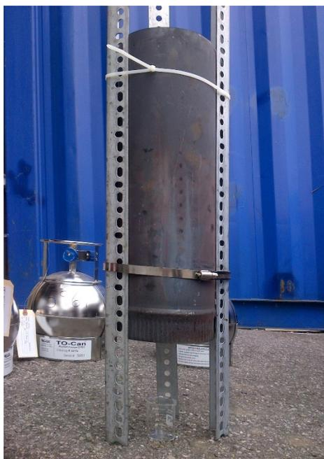
Figure 93: Stack assembly used in Herder/Torch Impingement tests
