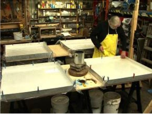
Figure 1: Lined 1-m<sup>2</sup> steel pans used for experiments.
