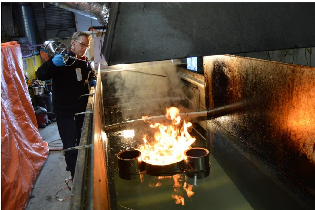
Figure 91: Mechanically contained oil burning
