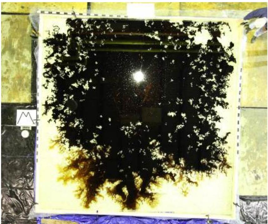
Figure 32: Oil spread to equilibrium thickness in slush ice.
