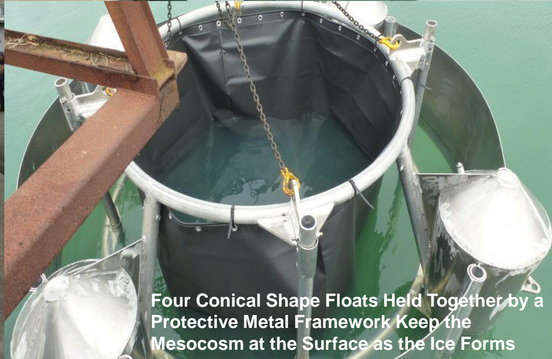
Mesocosm Buoyancy Testing at Cedre
