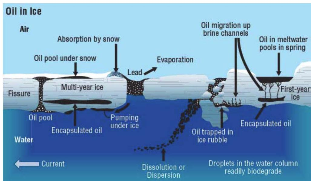
Figure 7. General fate of oil spilled under or on ice (Source: ExxonMobil).
