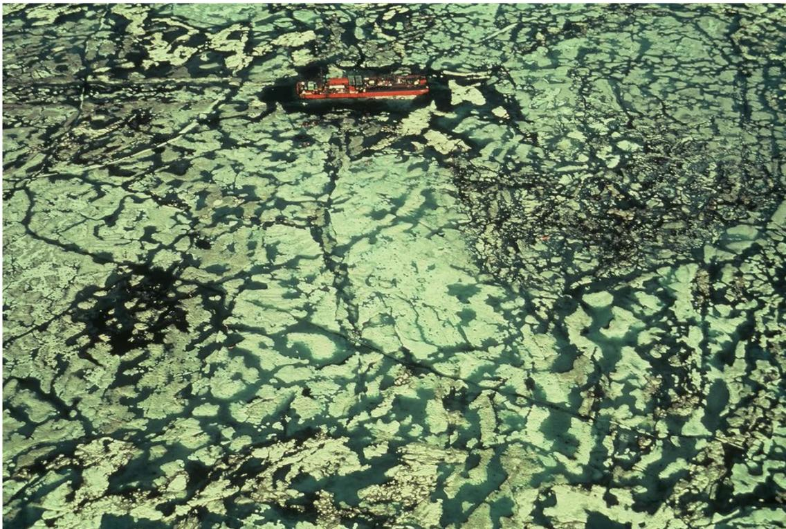
Figure 12. Oiled melt pools from subsea blowout under ice with 1-mm coverage surfacing in late spring (Source: D. Dickins).
