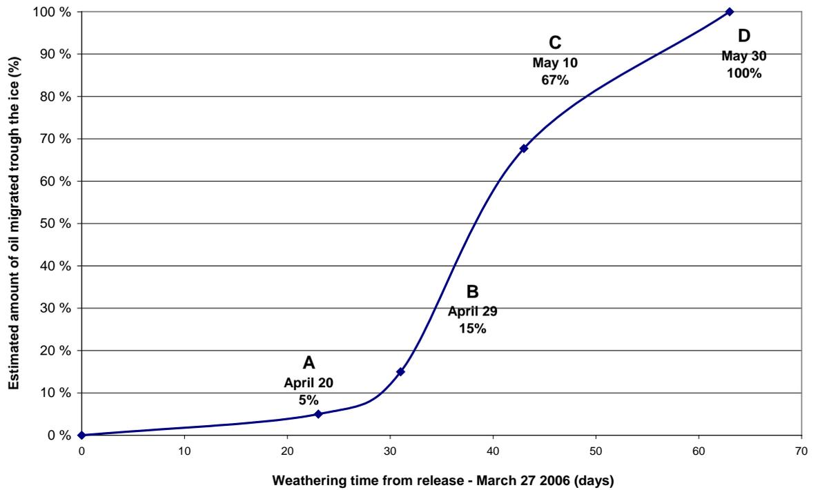
Figure 14. Exposure of encapsulated oil (Source: D. Dickins).
