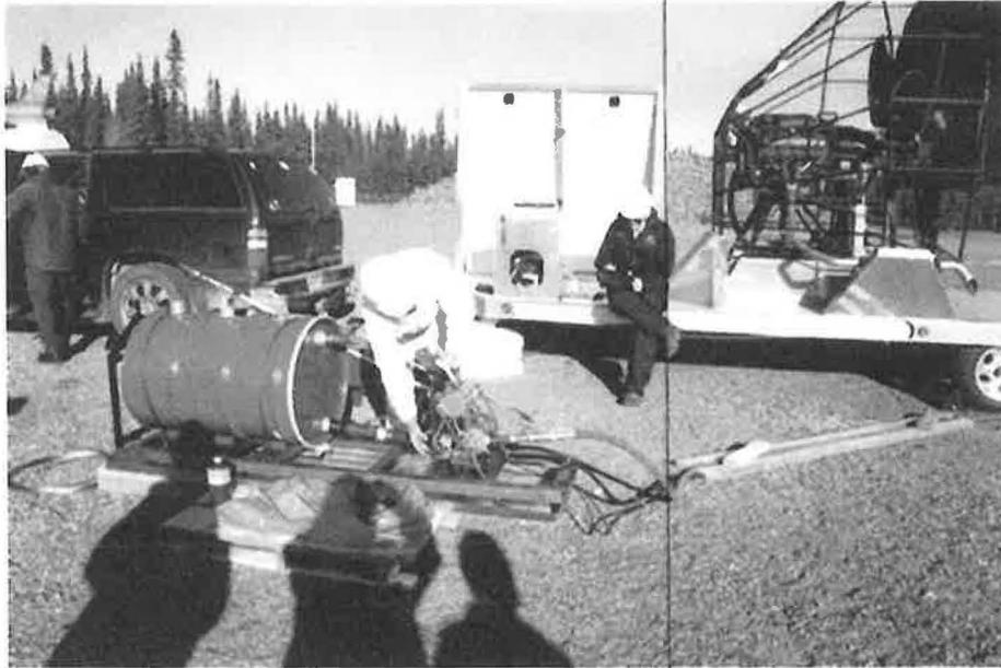
**Figure 4 – Modified Helitorch – Simplex Model 5400**
