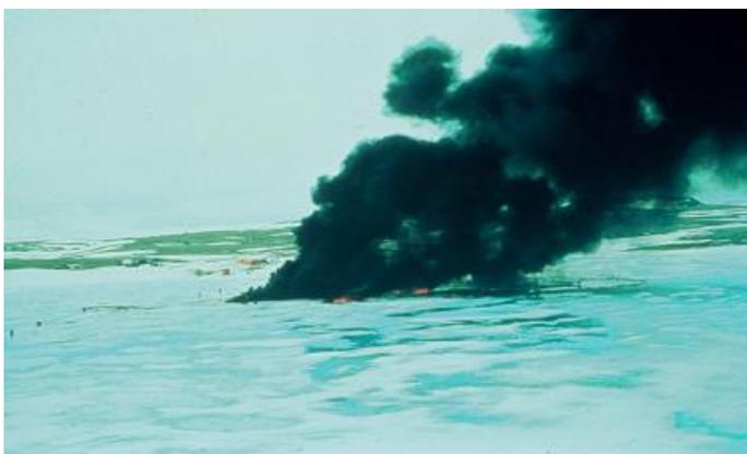
Figure 17. ISB at Balaena Bay experimental spill under ice (Source D. Dickins).
