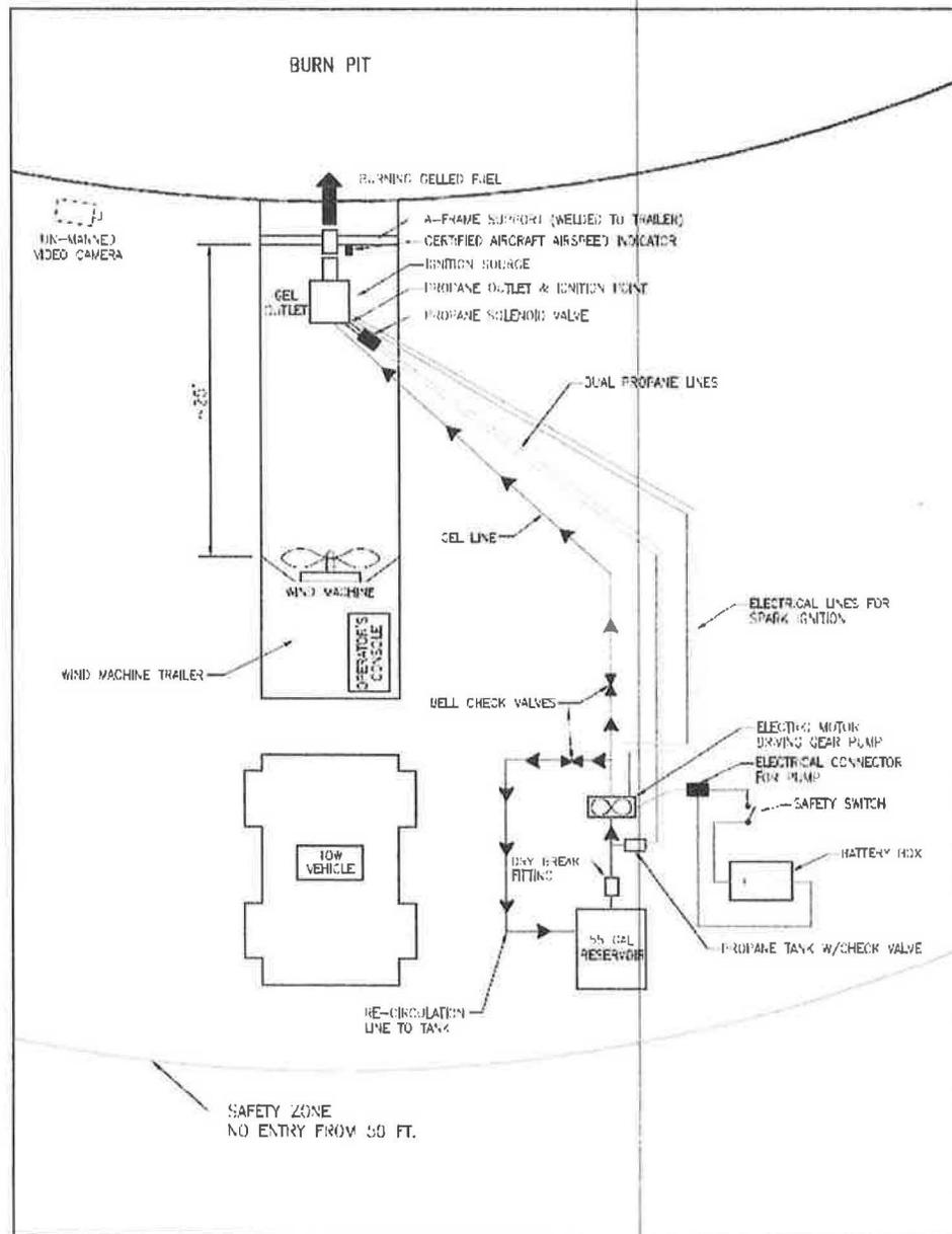
Figure 3 – Test Set-Up P&ID
