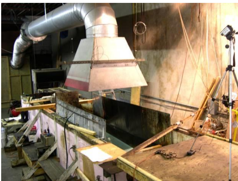
Figure 5. Wind/wave tank rigged for burn tests.
