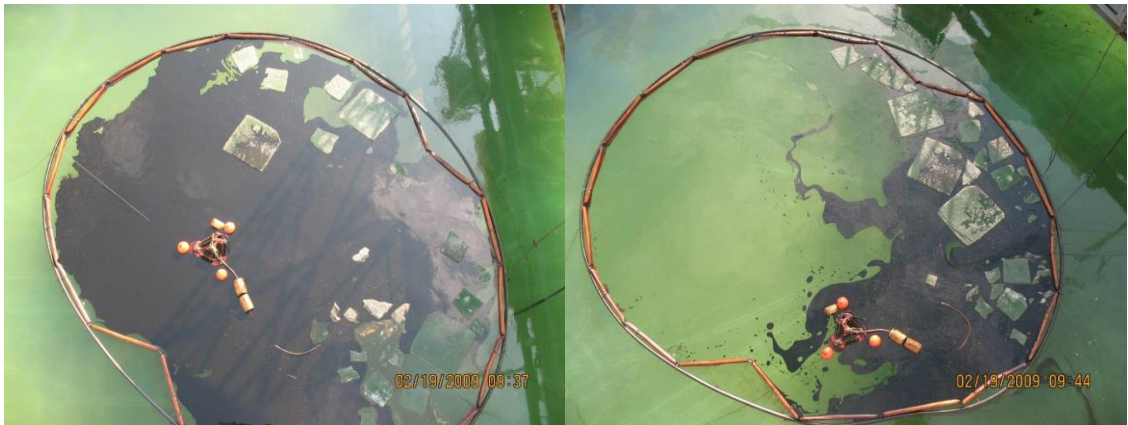
Figure 31. Overhead view of disc skimmer test with 10% ice before and after herding.
