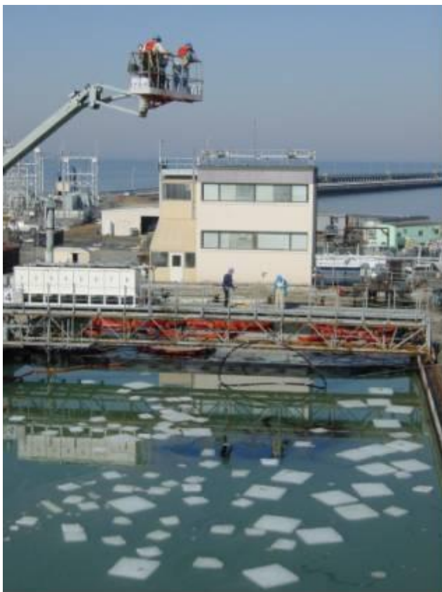
Figure 8. Herder test in drifting ice at Ohmsett.
