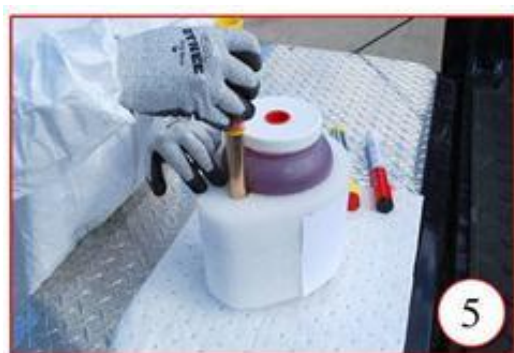
Figure 8 Safe Start hand-held igniter. (source: Elastec / American Marine)
