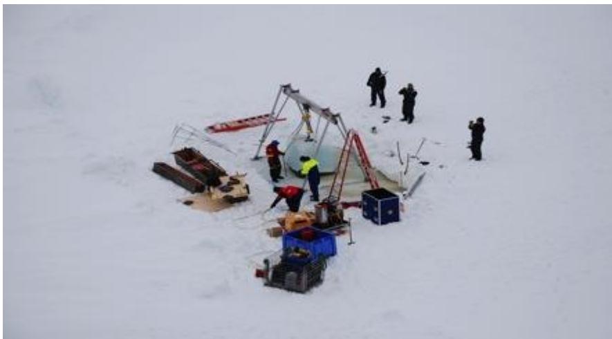
Figure 5.3 Example of a 1.5m x 1.5m x 1.5m hole cut in sea ice. The process associated with cutting this hole, from the time the gear was offloaded on the ice (in this case from an icebreaker) until the hole was cut and secured lasted ~6 hours. It involved setting up the gantry frame, drilling an augur into the ice to lift the ice block, using a hot water cutter to cut through and then pulling out the ice plug to provide access to the hole.
