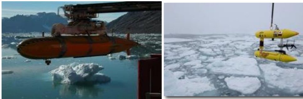
Figure 2.1.2 The Autosub AUV (left), a large (4m) torpedo shaped AUV and the smaller (1.5m) Jaguar AUV, a hover capable multihull design. Both have been used extensively for under-ice mapping missions
