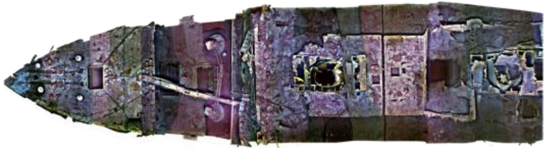
Figure 3.3.3 Individual images collected underwater mosaicked into a composite to obtain a global perspective. 866 images obtained by cameras on an ROV were combined in this rendering of the RMS Titanic.
