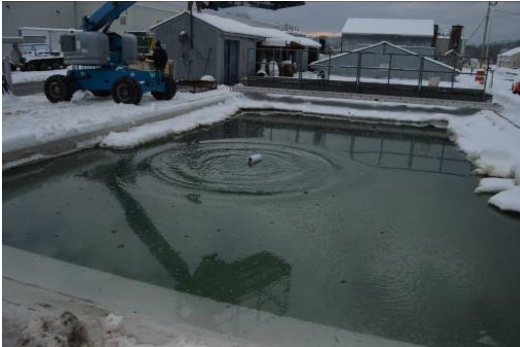
Figure 81 Activated igniter hitting water during pre-test
