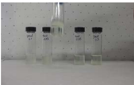
Figure 41. 15°C Diesel at 30 minutes with 0.20g gel
