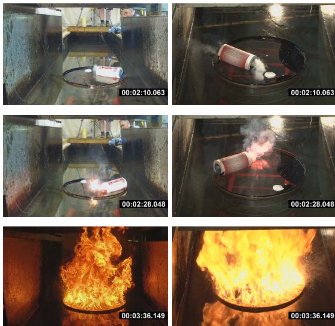
Figure 68. Test #12 Successful burn with Jet A1
