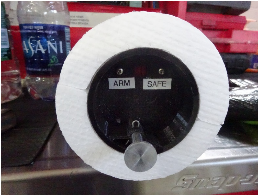
Figure 92. New CAD Igniter end cap
