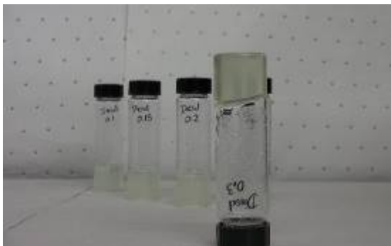
Figure 53. 15°C Diesel at 24 hours with 0.30g gel
