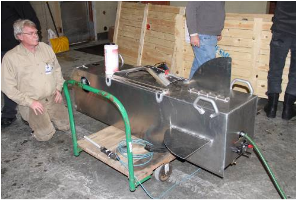
Figure 71 Integrated Igniter/Herder Application System with cover on
