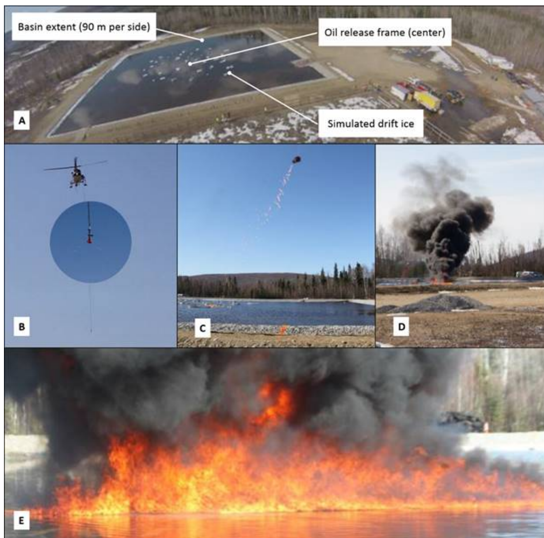
Figure 2. Field Test of Helicopter Herder Application and Crude Oil Ignition.
