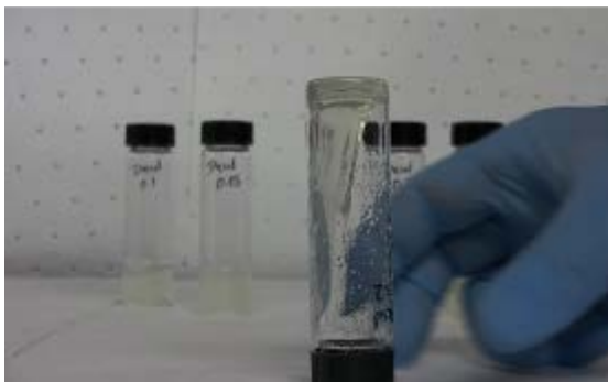
Figure 51. 15°C Diesel at 24 hours with 0.20g gel
