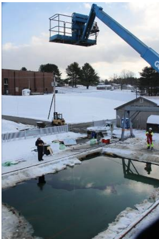
Figure 77 Positioning IIHAS on person-lift over herded slick
