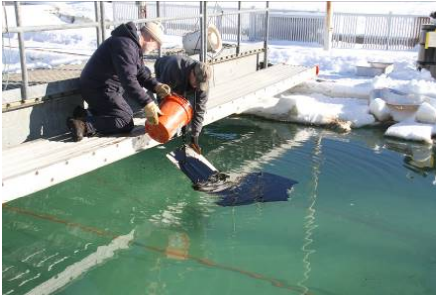
Figure 76 Spill plate to pour oil onto water surface
