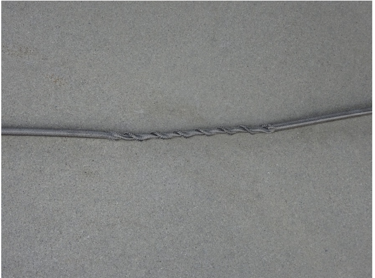
Figure 8770. Braided steel hose twisted during flight tests.
