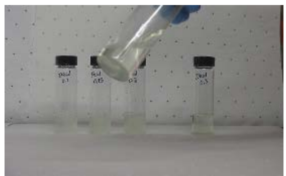
Figure 42. 15°C Diesel at 30 minutes with 0.25g gel
