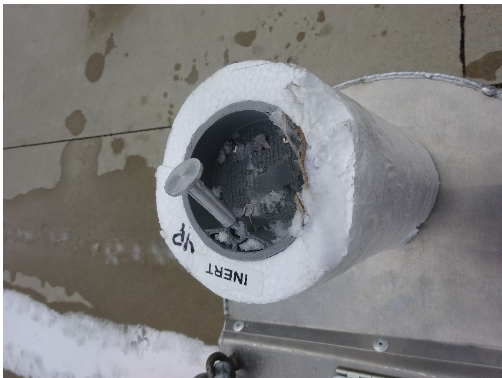
Figure 94. Damage to pin and cartridge
