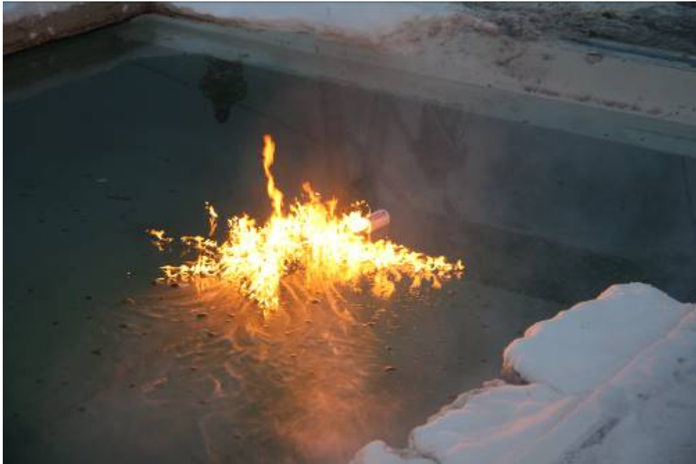
Figure 83 Gelled gas ignites 58 seconds after flare fired (2 minutes 52 seconds since release)
