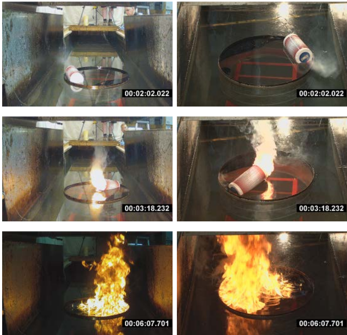
Figure 69. Test #13 Successful burn with premium gas
