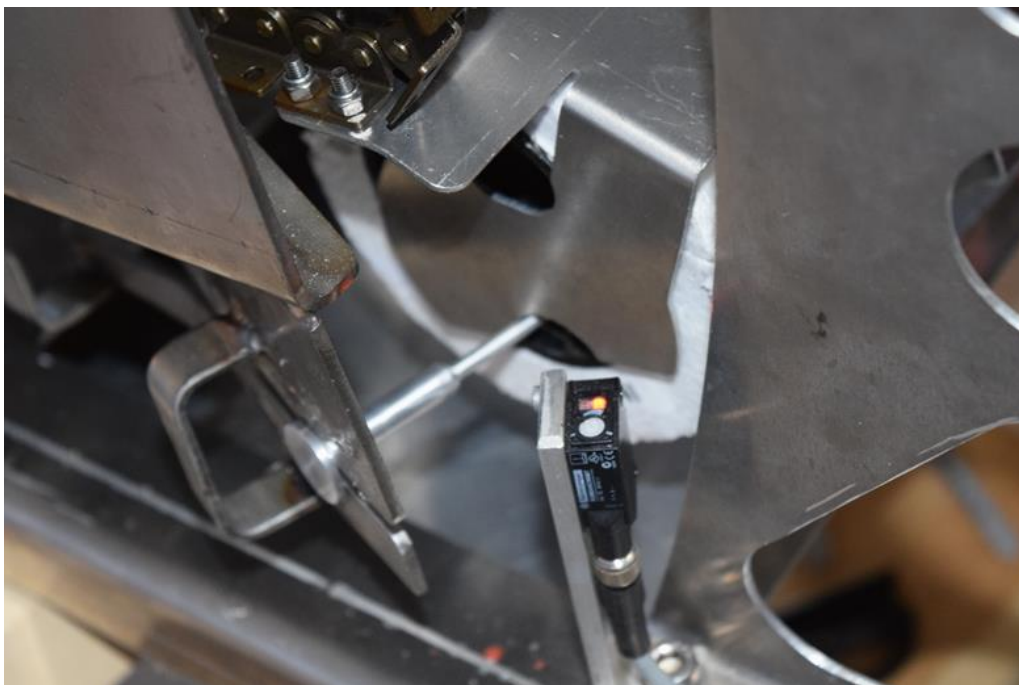
Figure 93. SIM with Jammed Igniter Cartridge
