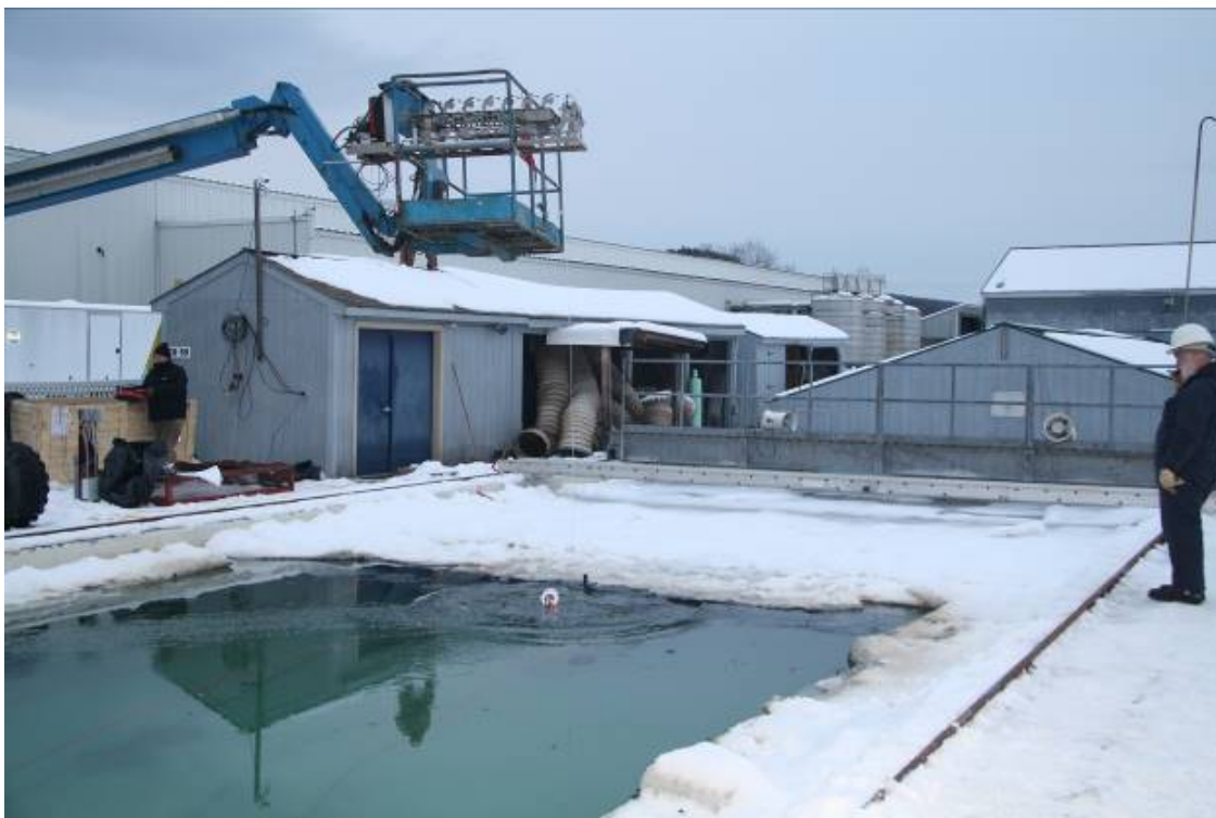
Figure 78. Igniter landing on slick
