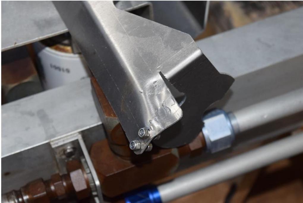
Figure 95. Damage to SIM from Jammed Cartridge
