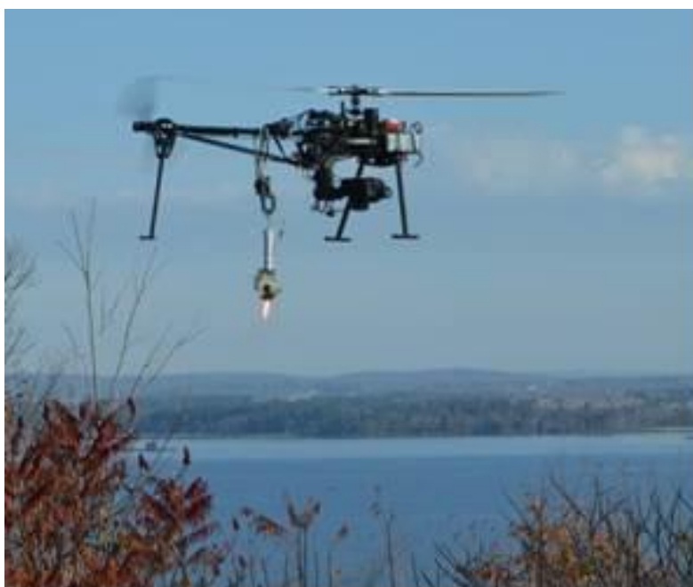
Figure 77: Responder triggering modified flare ignition
