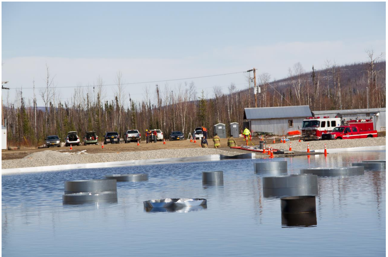
Figure 9: Sheet metal "faux" floes constructed to replace melting ice
