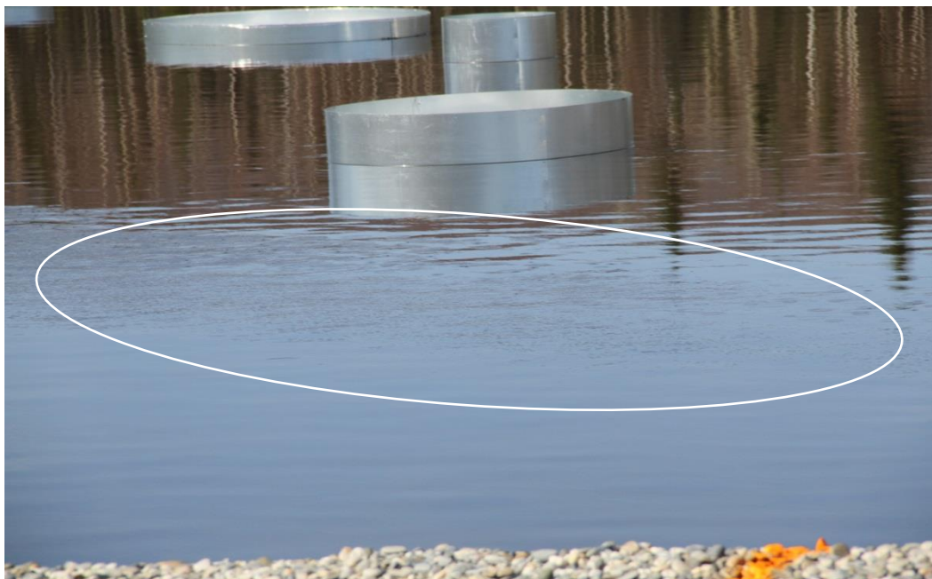
Figure 53: Herder laying on water surface after first application by helicopter (Test 4)
