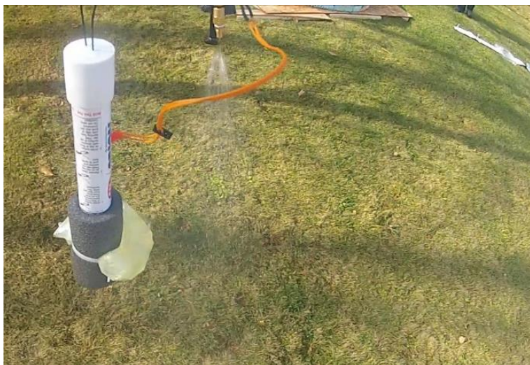
Figure 74: Herder being dispensed (igniter flare in foreground)
