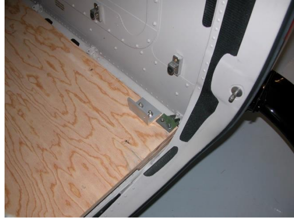
Figure 37: Rear seat belt attachment brackets
