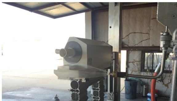
Figure 27: Flat Fan 8008 Nozzle with ThickSlick
