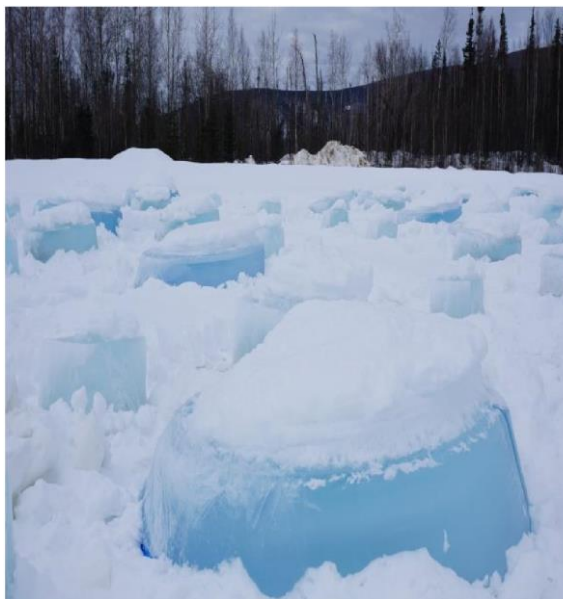
Figure B-15: Icebergs post form removal
