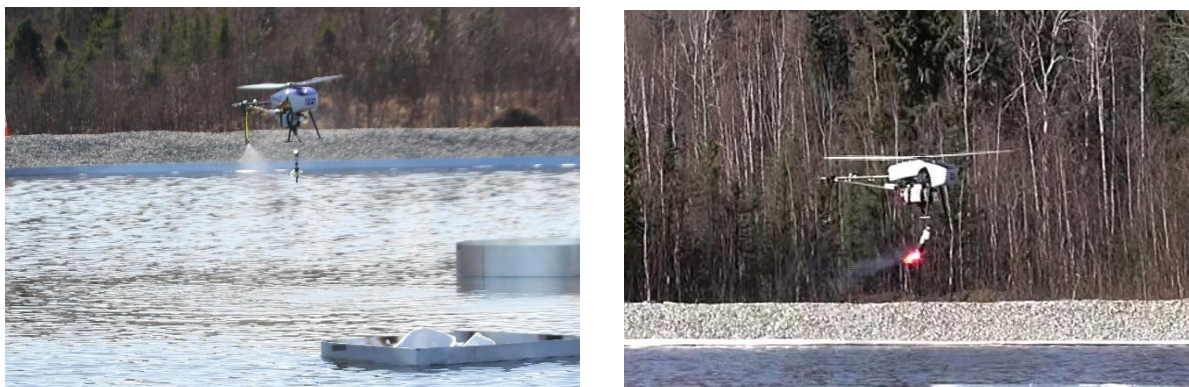
Figure ES-6: Responder UAV spraying simulated herder and carrying ignited flare
