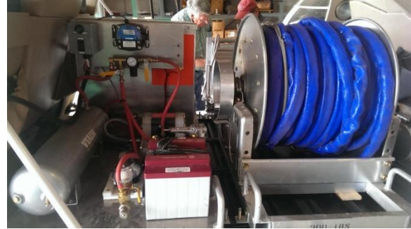
Figure 31: Herder Application System: Controls and Reel
