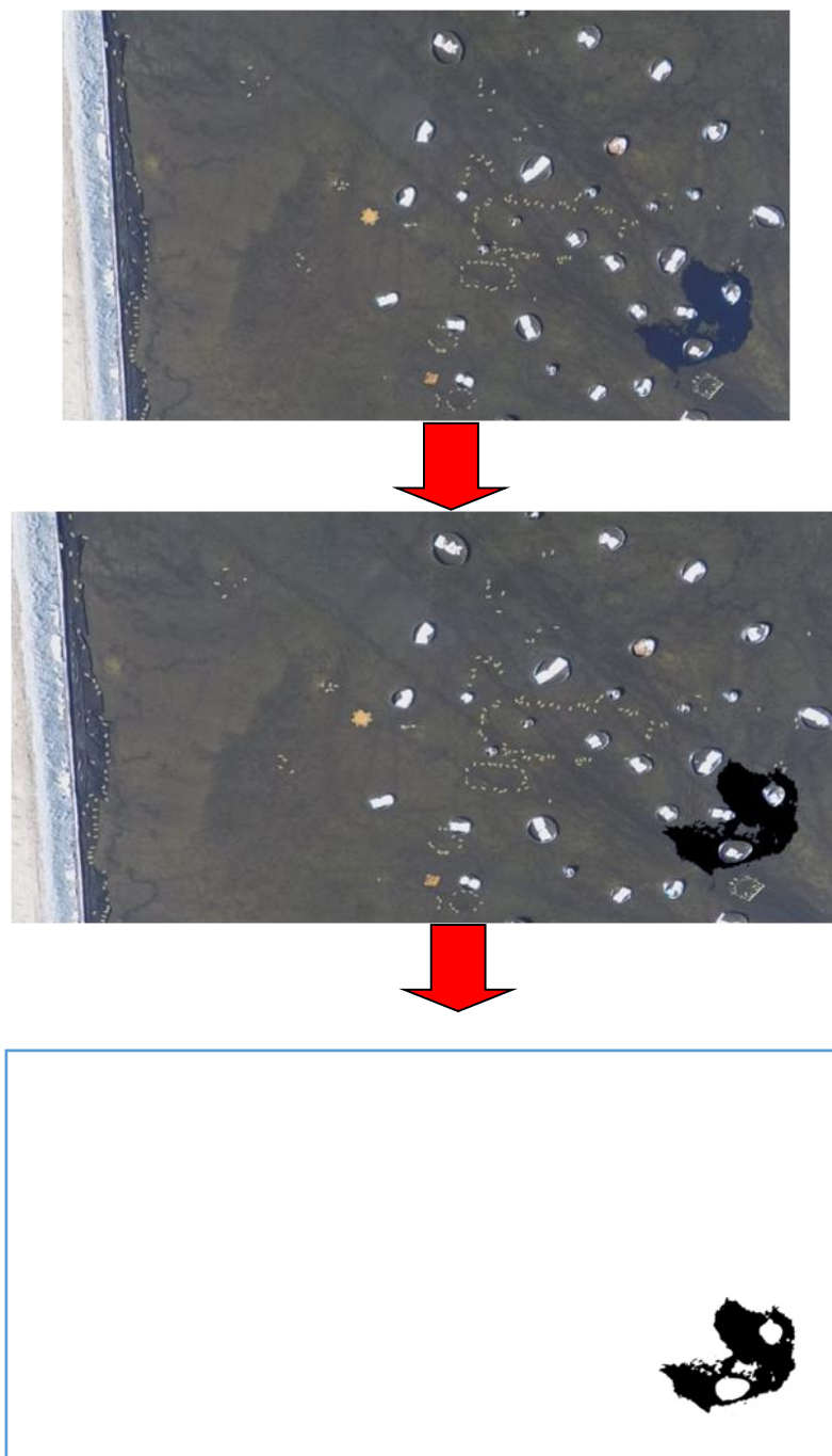
Figure 79: Digital transformation of aerial photographs to determine slick area
