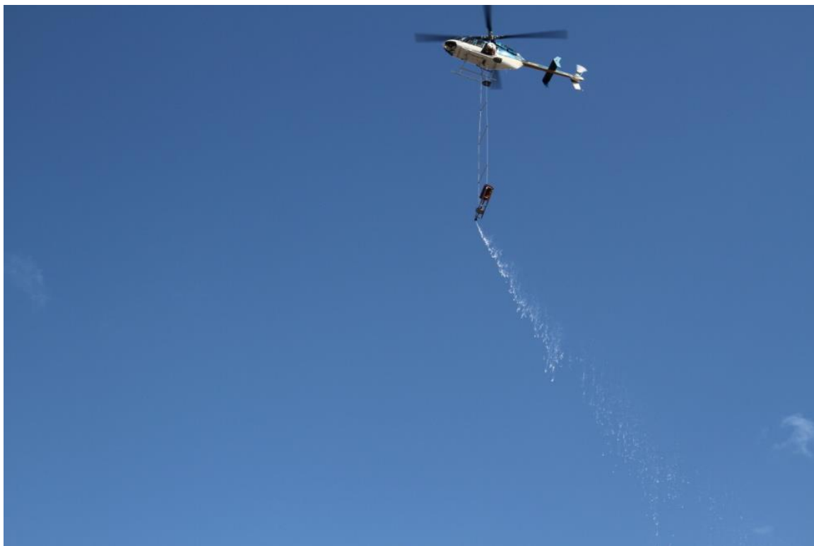
Figure 42: Diesel / gasoline mix failing to ignite from Heli-torch
