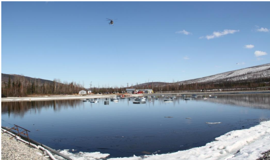
Figure 40: Helicopter applying herder (Test 1)
