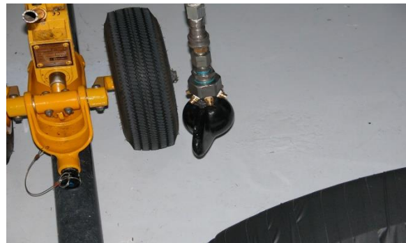
Figure 39: 5.5kg weight on end of nozzle
