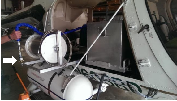
Figure 30: Herder Application System: Nozzle Assembly
