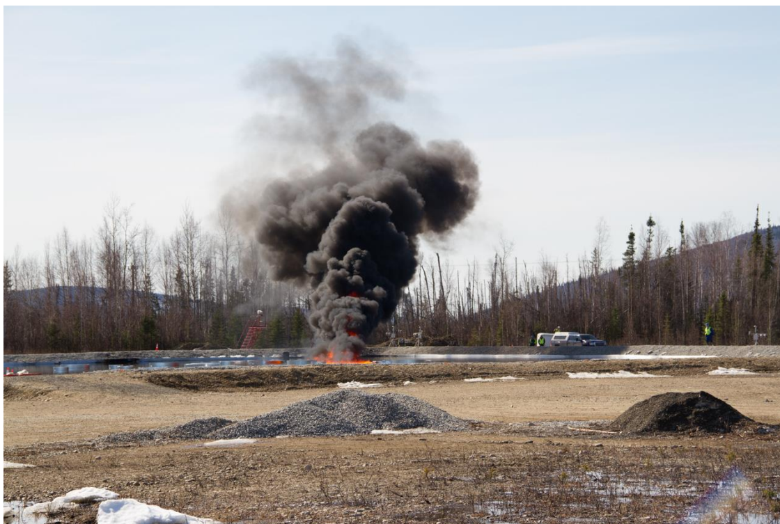
Figure 51: Slick burning in middle of basin (Test 3)
