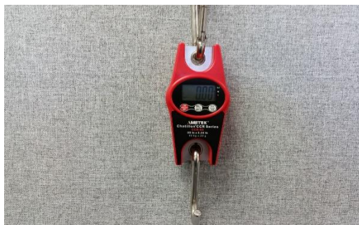
Figure 18: Digital Hanging Weigh Scale
