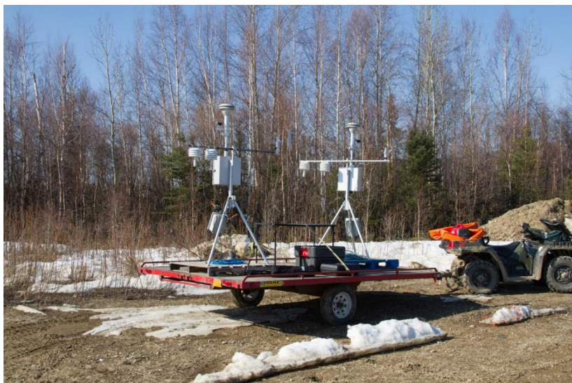
Figure 16: Trailer-mounted air samplers
