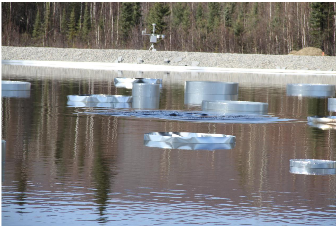
Figure 13: Release frame pulled off supports to release oil
