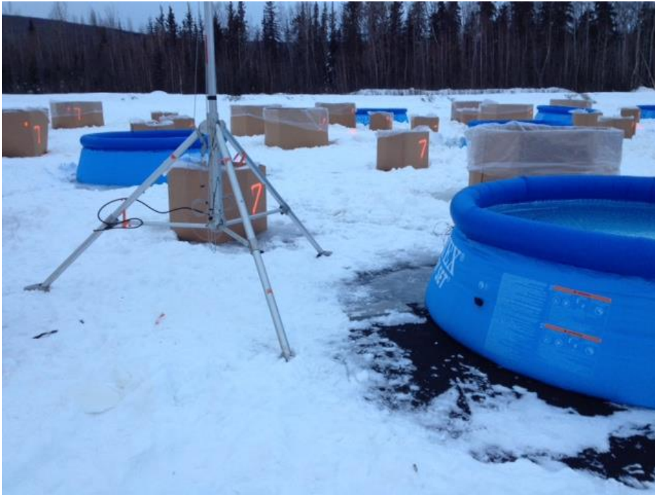
Figure 7: Cardboard boxes and children's pools used as forms to freeze water for ice floes
