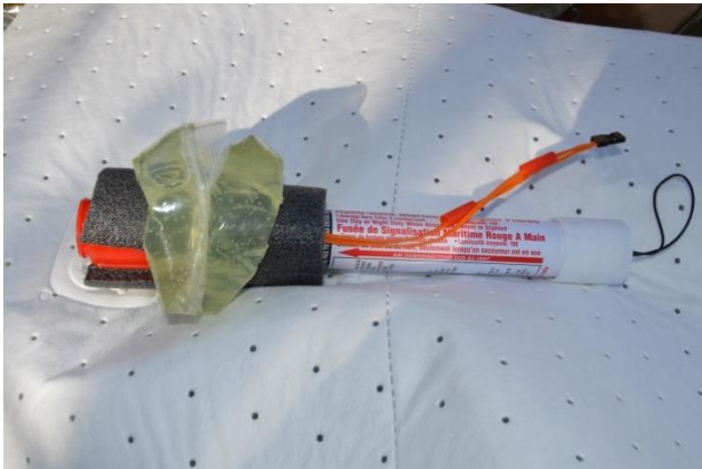
Figure 67: Marine Flare based Igniter System
