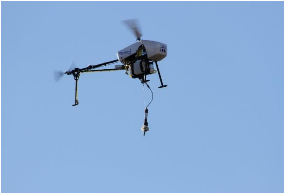
Figure 62: Responder UAV with Remote Igniter
