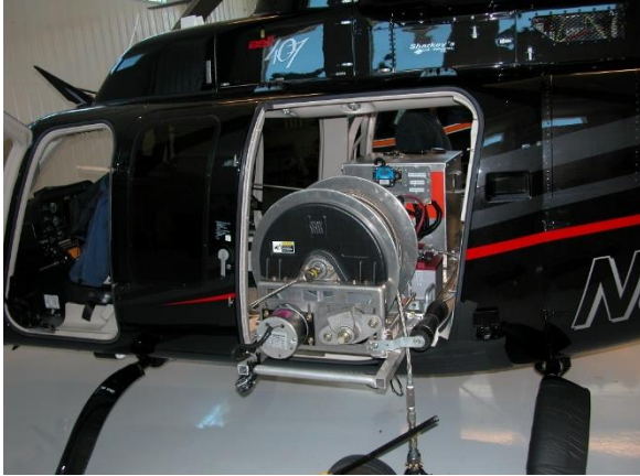
Figure 36: Hose reel extended out from helicopter
