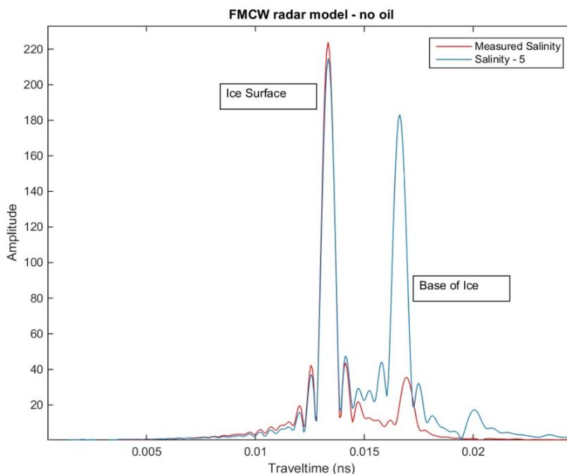
Figure 2 Modeled radar returns with the measured ice salinity during the January 2017 test (red), and with an ice salinity closer to the natural ice profile of Figure 1.
