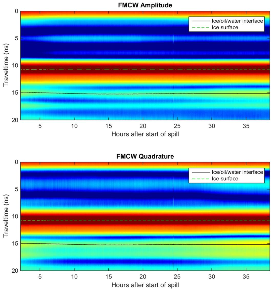
Figure 14 FMCW radar response from 2 hrs to 38 hrs after the start of the spill.
