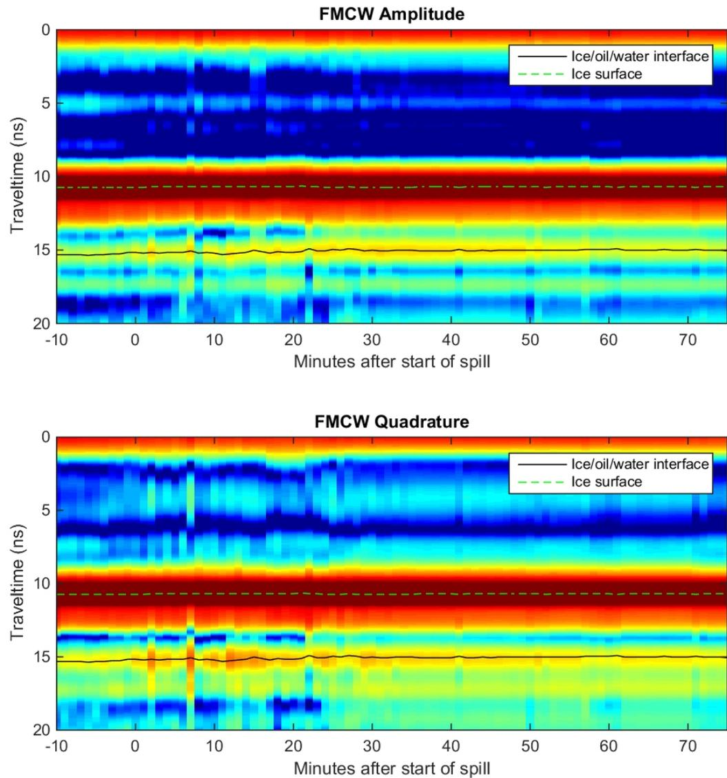
Figure 12 FMCW amplitude and out-of-phase (quadrature) component during and for a brief time after the injection.
