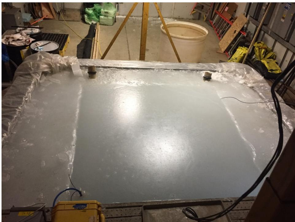
Figure 3 Photo of the prepared ice sheet prior to oil injection.
