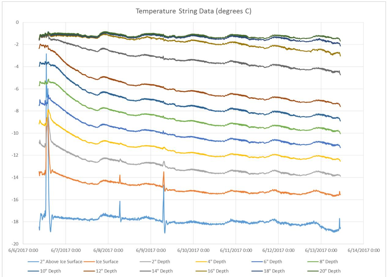
Figure 5 Ice temperature as a function of time and depth with the measurements beginning on the second day of radar testing and just prior to the oil spill.
