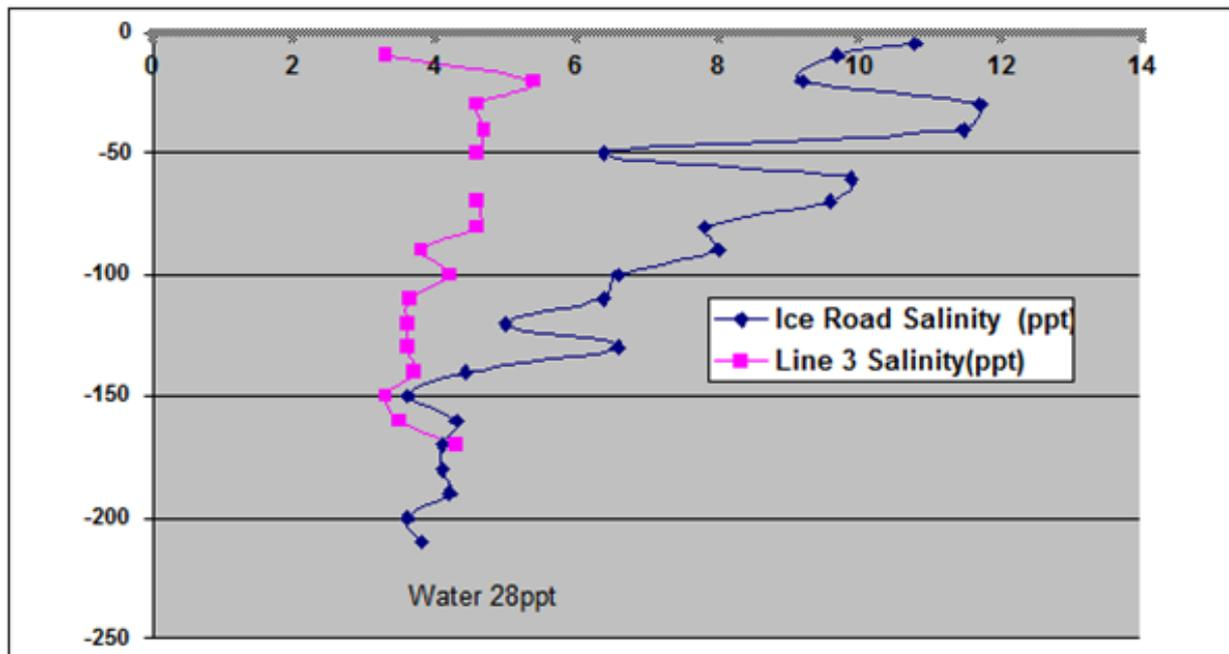
Salinities on the ice road (blue) are artificially high and similar to the salinities produced in the CRREL ice sheet during the January 2017 test. Radar signal could not penetrate the ice road. Salinities in the natural fast ice (pink) are roughly half that of the ice road through the central part of the ice sheet. Strong radar returns were observed from the base of the natural ice. (Figure courtesy of DF Dickins)
