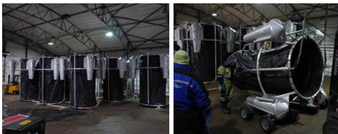
Figure 3 Assembly of the 8 mesocosms in Svea (source CEDRE)
