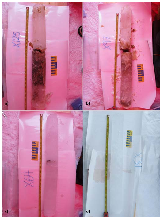
Figure 15 Example of cores collected at T3: a) Cude oil treatment, b) Oil+dispersant treatment, c) Burnt oil treatment and d) Control treatment
