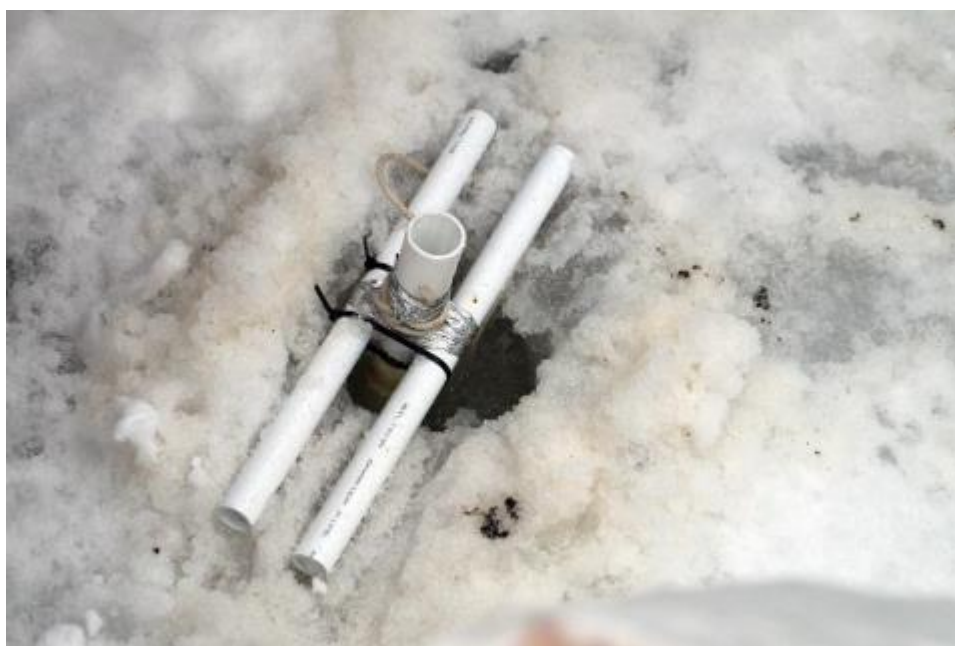
Figure 10 Outer tubing inserted in drill hole of mesocosm.
