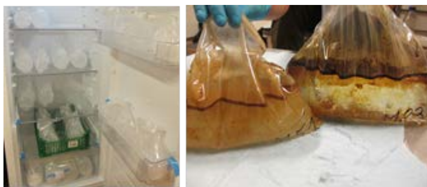
Figure 12 Ice core melting at 2-4 °C. Sterile bags containing melted ice cores from oil contaminated mesocosm (right bag), and from oil+dispersant mesocosm (left bag). Source: IRIS
