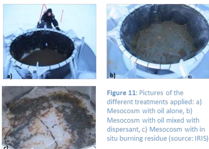
Figure 11 Pictures of the different treatments applied: a) Mesocosm with oil alone, b) Mesocosm with oil mixed with dispersant, c) Mesocosm with in situ burning residue (source: IRIS)
