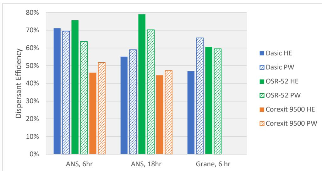
Figure B 4 Dispersant efficiency in 35 ppt salinity water for ANS and Grane crude oils (HE: High energy, PW: prop wash).
