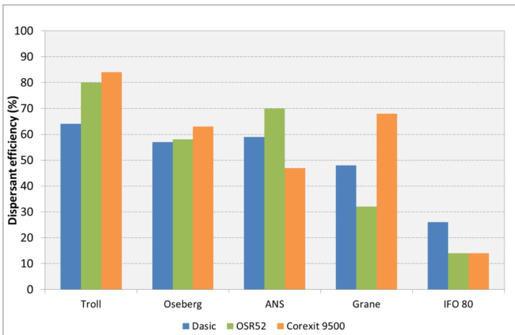
Figure 3.1 Dispersant efficiency vs dispersant type. Oils were weathered for 18 hrs in 80% ice and 35 ppt salinity water. DE measured from water grab samples collected after prop wash.
