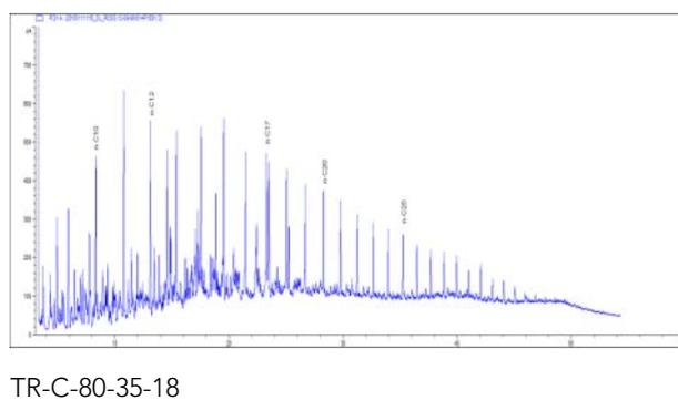
Figure D 4 GC chromatograms of Troll crude oil weathered for 18 hrs in the flume prior to dispersant testing. Explanation of test identifications is provided in Table 2.6.
