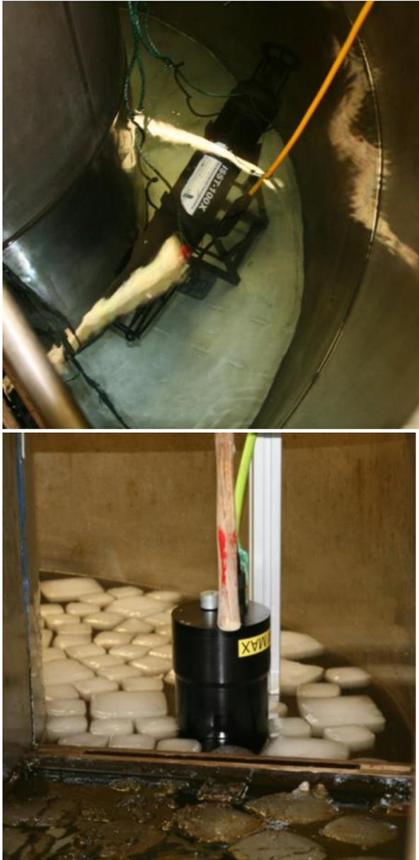
Figure 2.2 SINTEF flume prior to dispersion: LISST positioned horizontally at 50 cm depth (left) and SilCam positioned vertically with monitoring at 50 cm depth (right photo).
