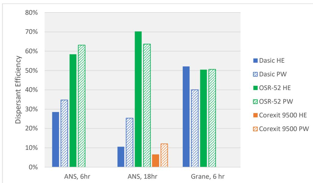
Figure B 5 Dispersant efficiency in 15 ppt salinity water for ANS and Grane crude oils (HE: High energy, PW: prop wash).
