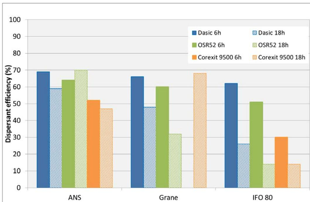
Figure 3.2 Dispersant efficiency vs weathering time. Oils were weathered for 6 hrs or 18 hrs in 80% ice and 35 ppt salinity water (Grane Corexit 9500 6hrs not performed). DE measured from water grab samples collected after prop wash
