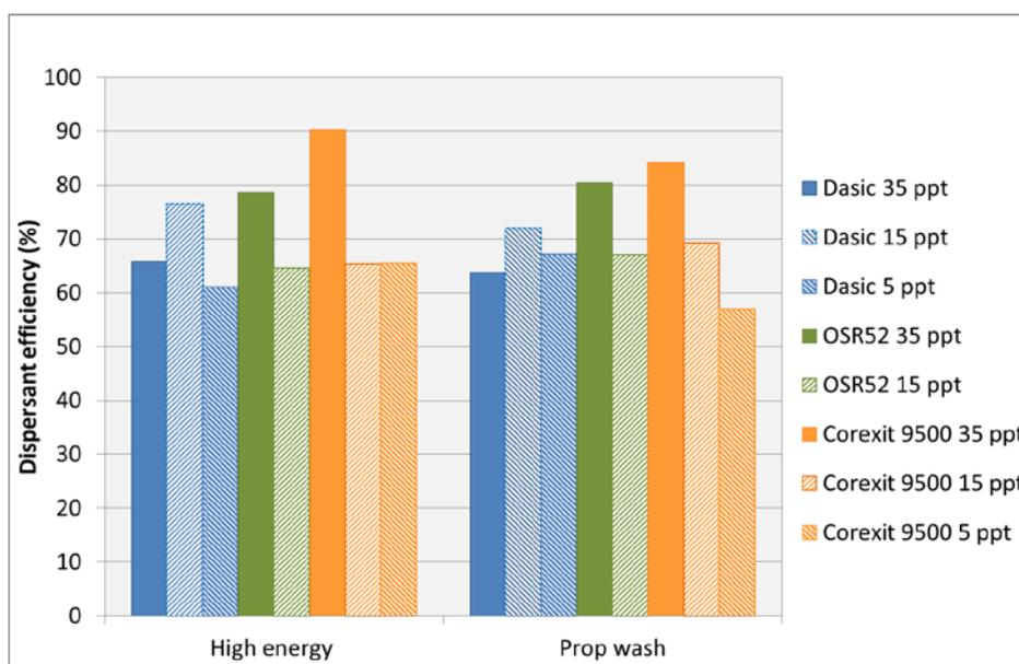
Figure A 1 Dispersant efficiency for Troll Blend
