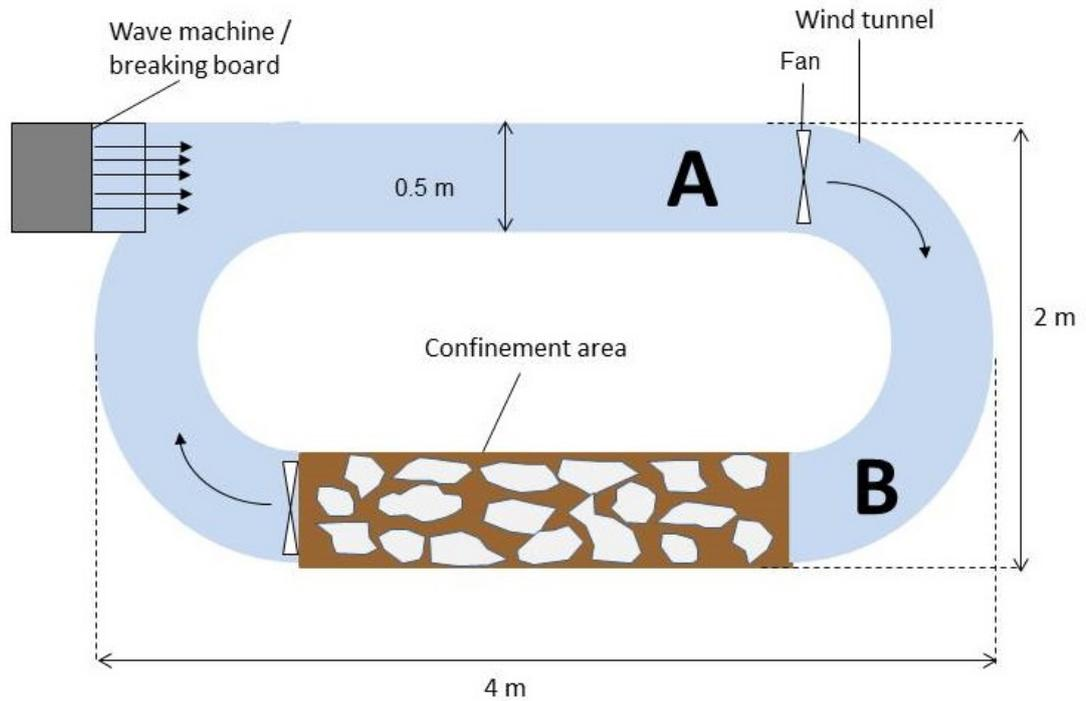
Figure 2.1 Sketch of the SINTEF and SL Ross flume
