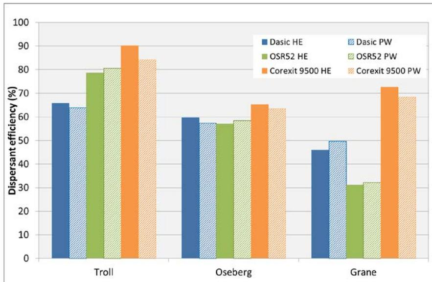
Figure A 4 Comparing dispersant efficiency in 35 ppt salinity water for the three oil types (HE: High energy, PW: prop wash).
