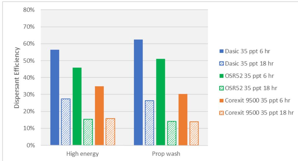
Figure B 3 Dispersant efficiency for IFO 80
