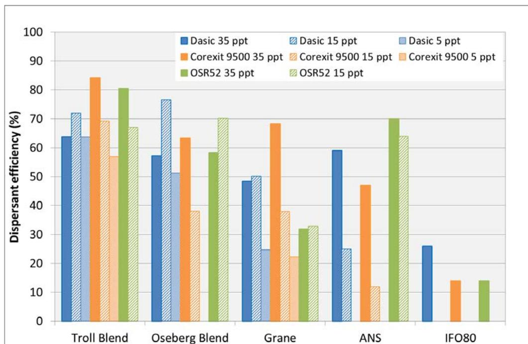
Figure 3.3 Dispersant efficiency vs water salinity. Oils were weathered for 18 hrs in 80% ice. DE measured from water grab samples collected after prop wash. No bars indicate that no testing was performed.
